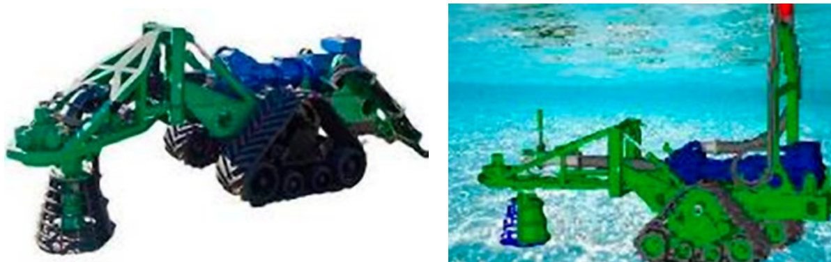
Figure 50. OSBORS unit used to retrieve oil from the bottom (Source: NOAA, 2013)
