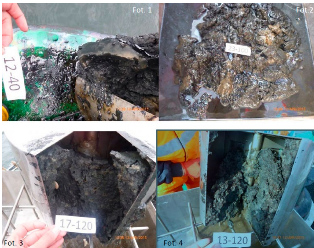
Figure 37. The content of the sampler collected at sites in the vicinity of the Stuttgart wreck in April 2016. At sites where heavy oil was macroscopically detected, no macrozoobenthos was found (photo 1 and 2), whereas macrozoobenthos was found in two remaining samples (photo 3 and 4) (Source: Maritime Institute in Gdańsk)
