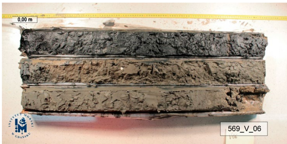
Figure 31. Sample core after preparation for geological analysis, before sampling for chemical analysis (Source: Maritime Institute in Gdańsk)
