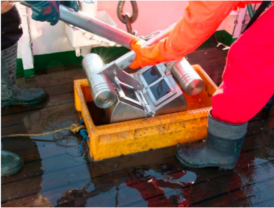
Figure 28. Van Veen sampler during work on board R/V IMOR (Source: Maritime Institute in Gdańsk)
