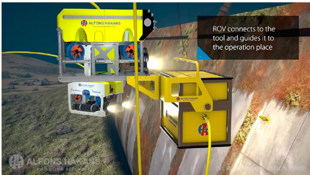
Figure 32. ROV with Hot Tapping device produced by Alfons Håkans (Estonia and Park Victory cases info 2015-12-08 KR.pdf)
