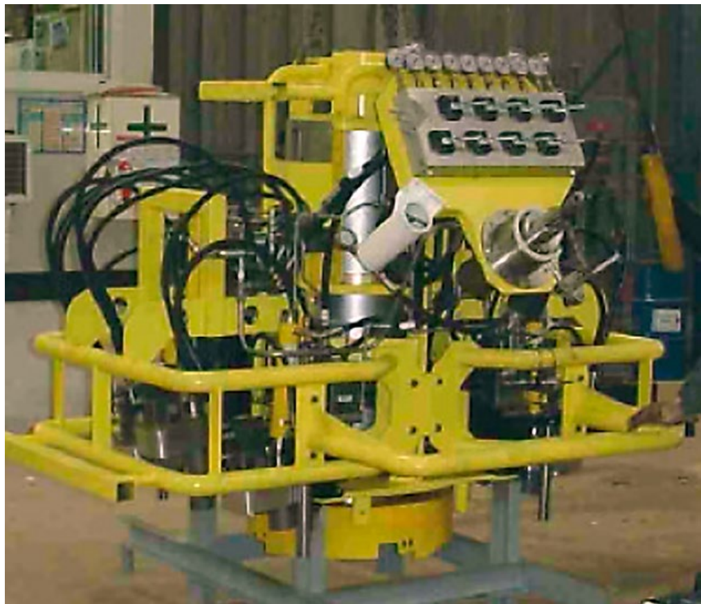
Figure 31. Hot-tapping device used at Prestige wreck
